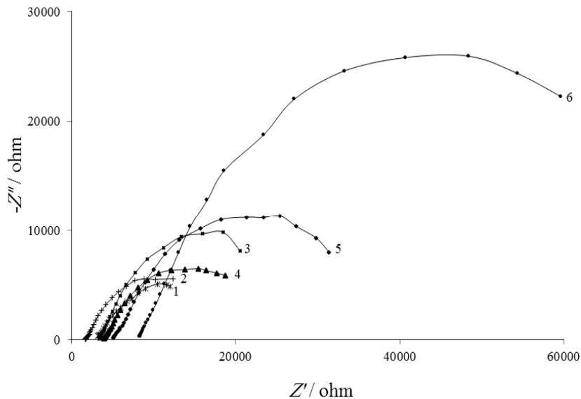
**Fig. 2.** Nyquist diagrams of aluminum alloy electrode in 100 ppm NaCl and ethylene glycol-water solution with different concentrations of ethylene glycol: 1: 0; 2: 10; 3: 20; 4: 30; 5: 40; 6: 50% V/V ethylene glycol solution.
