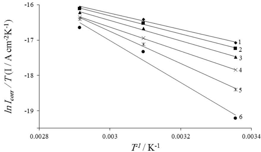
**Fig. 8.** Typical Arrhenius plots of  $\ln(I_{\text{corr}}T^{-1})$  vs.  $T^{-1}$  for aluminum alloy in 100 ppm NaCl at different concentrations of ethylene glycol: 1: 50; 2: 40; 3: 30; 4: 20; 5: 10; 6: 0% V/V
