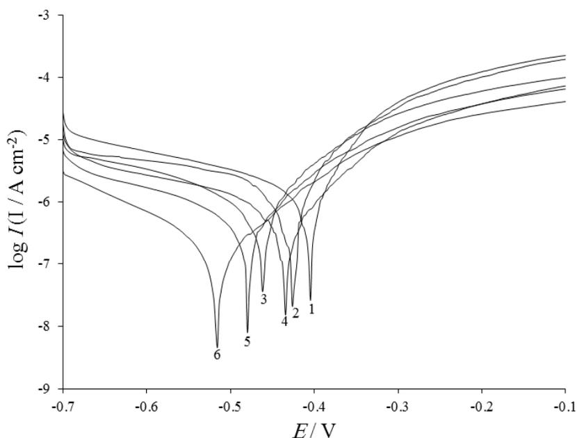
**Fig. 1.** Polarization curves of aluminum alloy electrode in 100 ppm NaCl and ethylene glycol-water solution with different concentrations of ethylene glycol: 1: 0; 2: 10; 3: 20; 4: 30; 5: 40; 6: 50% V/V ethylene glycol solution.
