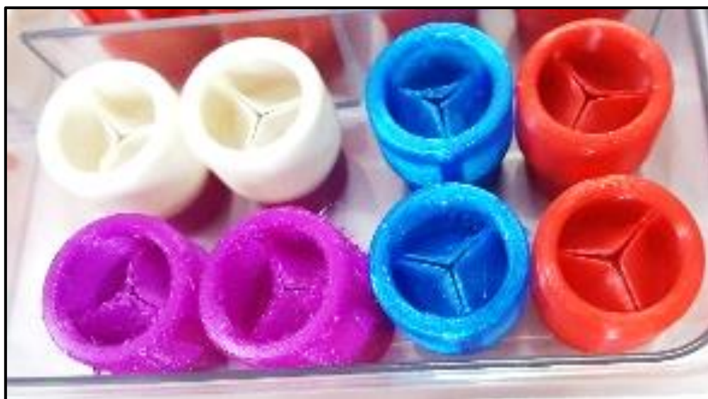
Fig. 9. The 3D printing of artificial mitral tri-leaflet mechanical heart valve
